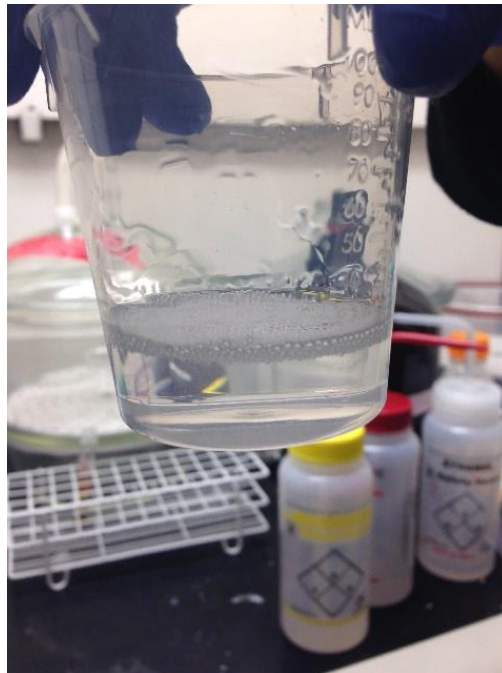
Figure B.4. Intermediate condition after 15 minutes of vacuuming.
