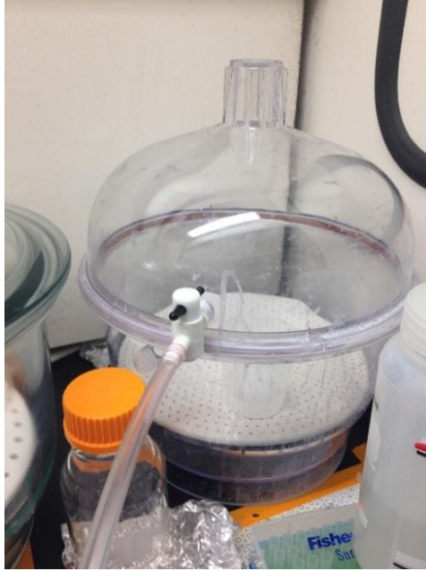
Figure B.3. Vacuum desiccator used to eliminate bubbles.
